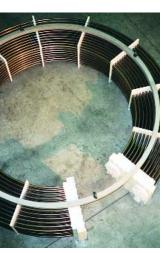
ITT Standard uses an integral finned tube to assure the highest efficiency, long life and reliability of service. The continuous helical fins are radially extruded from thick walled aluminum tubes in a cold rotary process. The result is an extremely rigid fin structure that is easy to maintain and has no possibility of loosening from the parent tube with a resulting loss in thermal performance. In similar fashion, corrosion at the fin interface is eliminated thereby promoting long coil life.
